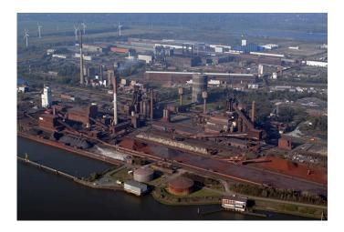
ArcelorMittal Bremen GmbH is one of the four German locations of ArcelorMittal Group. More than 3.500 employees produce more than 3,5 million tonnes of crude steel per year. The products range from slabs and hot rolled coils up to galvanized coils and laser welded blanks.
